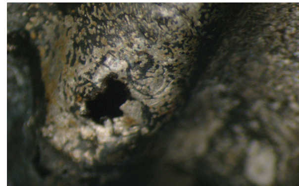
Stereomicroscope photo taken by Goodson Engineering of CSST perforation caused by lightning.
