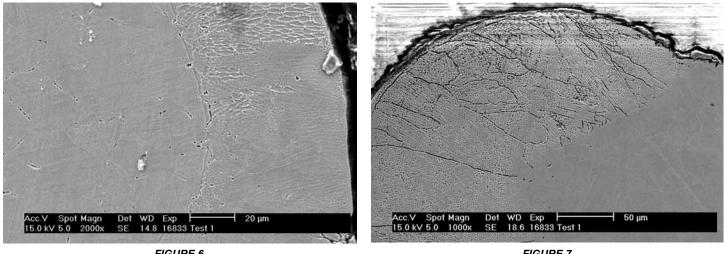
FIGURE 6 Sensitized CSST (1350 °F/732 °C) Normal equiaxed grains in CSST (left), re-solidified CSST microstructure (right)
