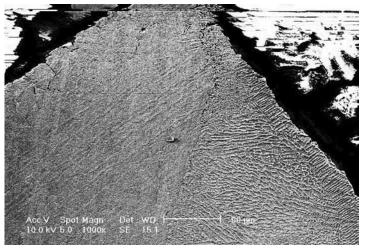
FIGURE 10 SEM micrograph of electrically induced hole after corrosion exposure Normal equiaxed grains in CSST (left), re-solidified CSST microstructure (right)
