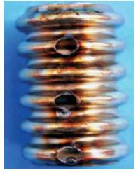
FIGURE 2 Ablation caused by electrical arcing.
