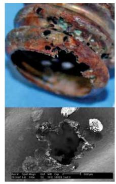
FIGURE 9 Corrosion induced hole
