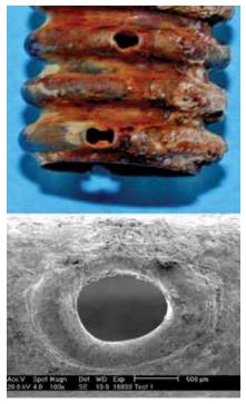
FIGURE 8 Electrically induced hole
