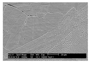
FIGURE 5 Normal equiaxed grains in CSST (upper left), re-solidified CSST microstructure (lower right)
