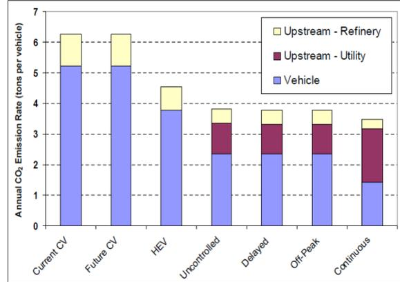
Figure 19: Net Vehicle CO<sub>2</sub> Emissions Rates
