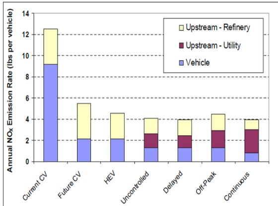
Figure 17: Net Vehicle NO<sub>x</sub> Emissions Rates
