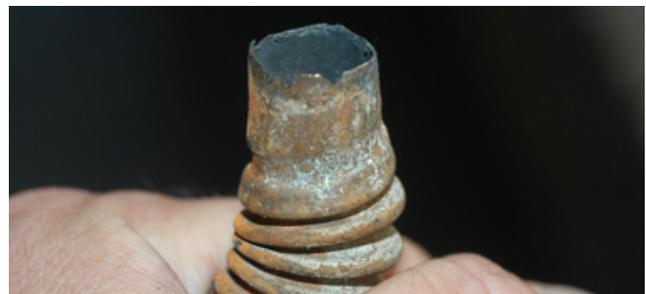
**Photo 2- arced end of a failed GAC**
