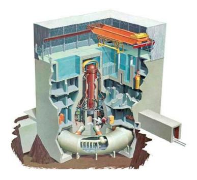
The first line of defense against any radiation release is the stainless steel *reactor vessel*. This is the copper-colored vessel in the center of the diagram. It houses the reactor core. The second line of defense is the *reactor*
