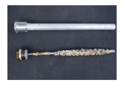
The resistor fails and the anode rod is nonLeaving the tank
