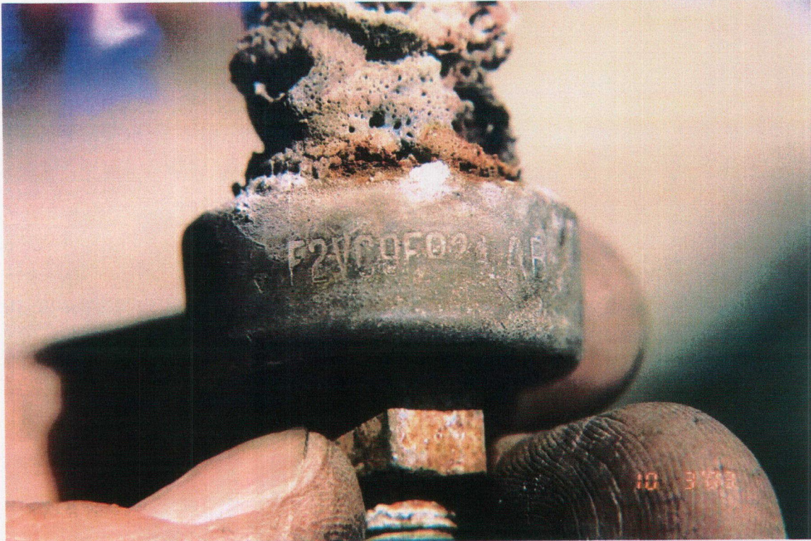
Remains of damaged switch found at scene
